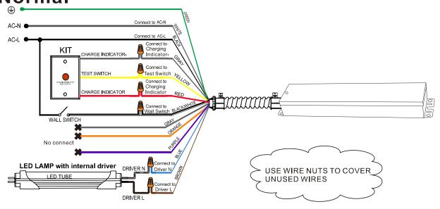
\*When the led driver power more than the emergency power B)With Dimmer
