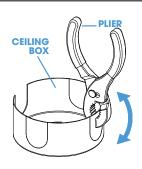
Remove the two pre-removable metal sheets on opposite sides of the ceiling box using pliers
