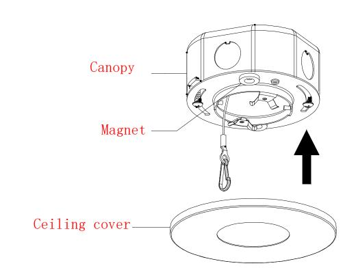
3Mount the steel rope onto the ceiling bracket
