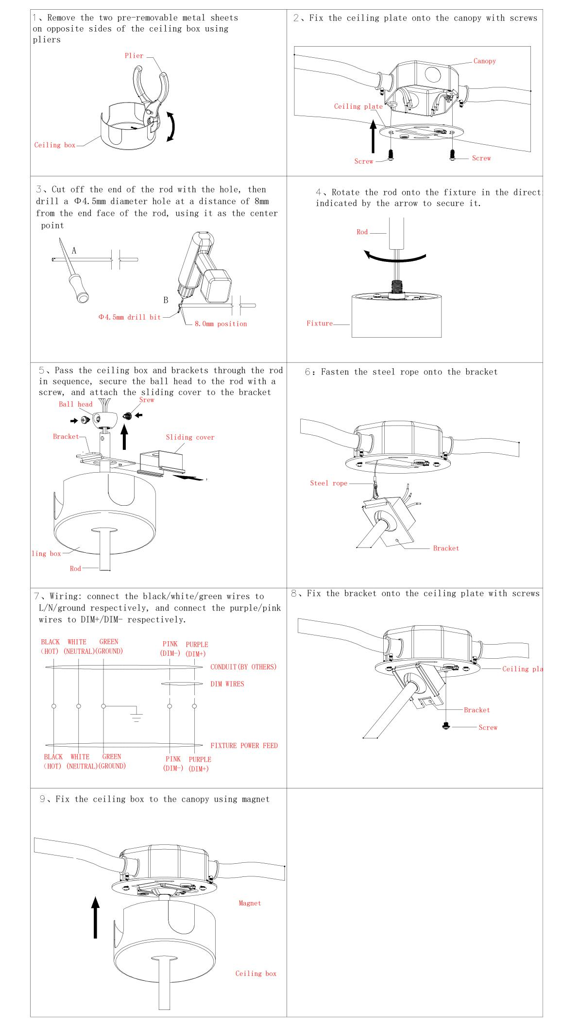
1. Remove the two pre-removable metal sheets on opposite sides of the ceiling box using pliers
