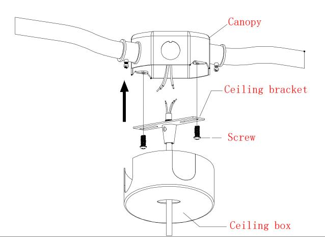
4. Wiring: connect the black/white/green wires to L/N/ground respectively, and connect the purple/pink wires to DIM+/DIM- respectively.
