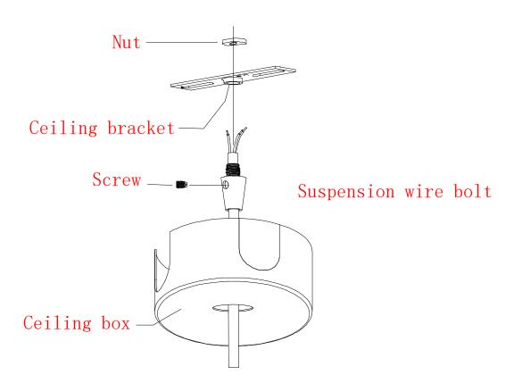
3. Fix the ceiling bracket to the canopy using screws
