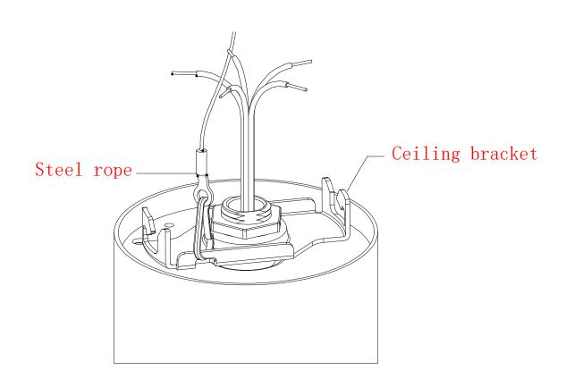
4Wiring: connect the black/white/green wires to L/N/ground respectively, and connect the purple/pink wires to DIM+/DIM- respectively.
