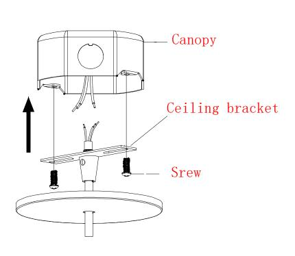
3. Wiring: connect the black/white/green wires to L/N/ground respectively, and connect the purple/pink wires to DIM+/DIM- respectively.
