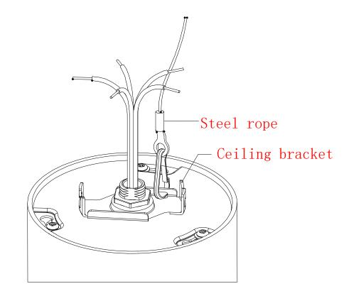
5. Wiring: connect the black/white/green wires to L/N/ground respectively, and connect the purple/pink wires to DIM+/DIM- respectively.
