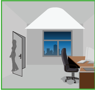
The light dims to "stand-by level" after hold time.
